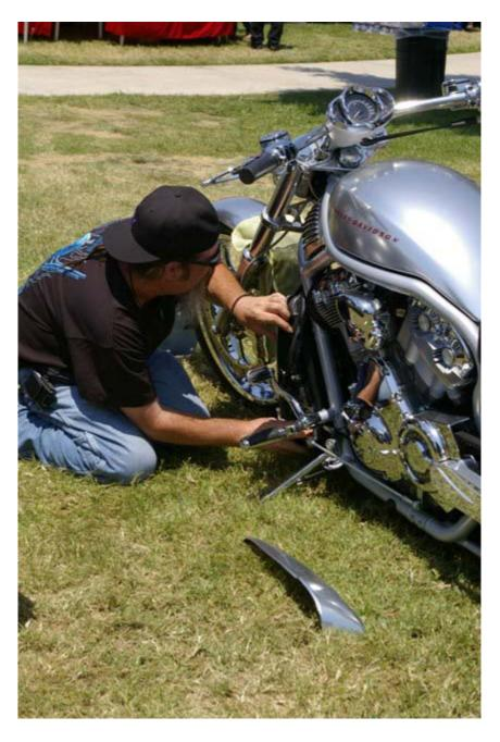
4. Now remove the bezels from the radiator cover by removing the three 10mm nuts. Then remove the two Phillips screws. Repeat this process for the other side. (Time out for more water.)
