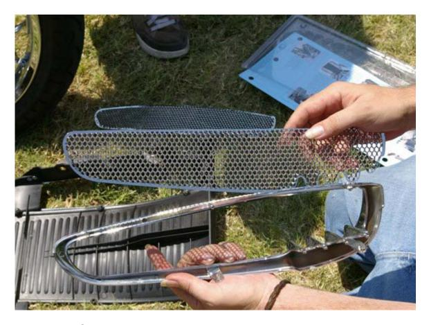
6. Install the Grilles between the chromed inlet bezels and the radiator cover. The fit is exactly correct so will slip in easily.
