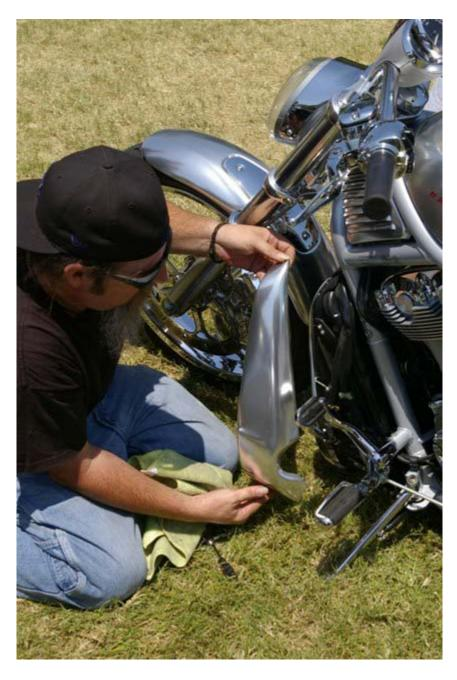
8. Re-install the side covers basically following the disassembly steps in reverse. Again, using thread locking compound. Then re-attach the wires to the left side cover and slide brake reservoir back into place.
