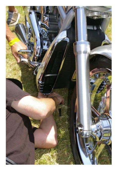
2. Remove side-covers by removing two tork screws found underneath the radiator housing. Pull out the bottom and lift on top, then repeat for the other side of the radiator, removing that cover. Place screws in safe container.
