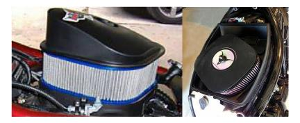
Now you have the necessary clearance for the Phantom Cover to be mounted the same way the stock air box cover mounts.
