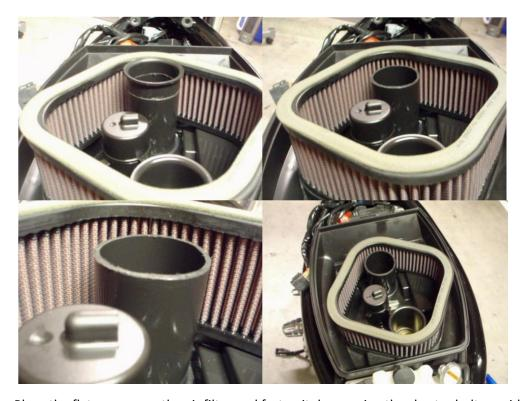
Place the flat cover over the air filter and fasten it down using the shorter bolt provided and your factory thumb
