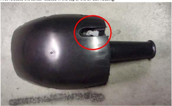
Unclip the sensor from the top housing unit and clip on to female port. Leaving the sensor unplugged will cause the engine light will remain on.
